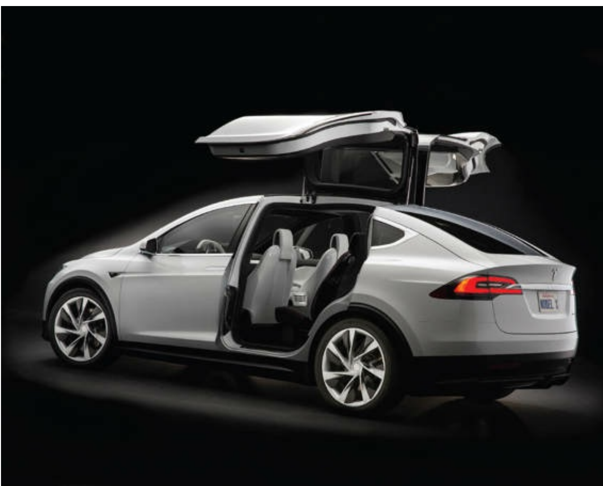
Tesla's next car will be the Model X SUV with its signature "falcon-wing doors." Photograph courtesy of Tesla Motors
